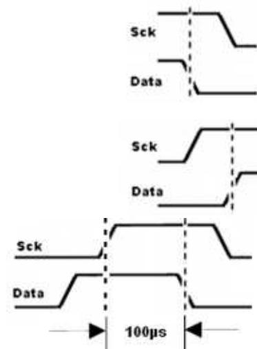
The serial interface of the HTG3800 Series W/O TC modules is optimized for sensor readout and power consumption. HTG3800 W/O TC Series modules communication bus is very close to I2C bus for wiring and voltage levels. Start and stop signals are I2C compliant but:
