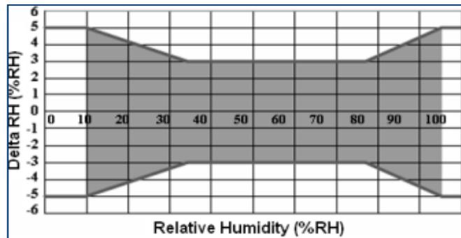
HTG3800 Series W/O TC modules are specified for maximum accuracy measurements within 10 to 95 %RH.
